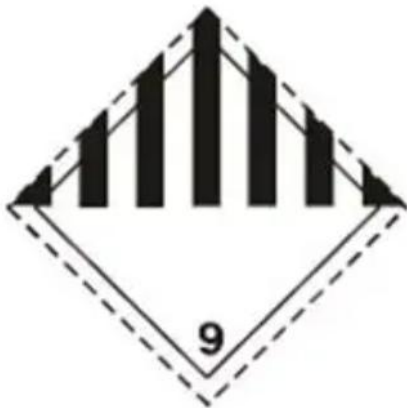
Figure 3 Class 9 hazard label
