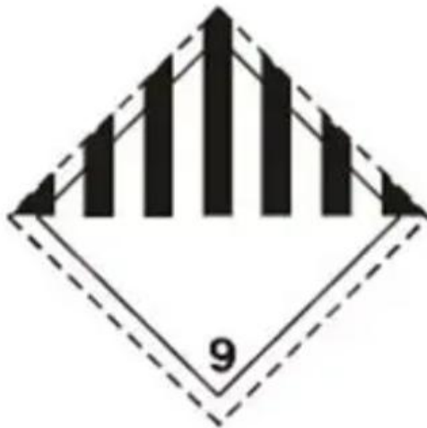
Figure 3 Class 9 hazard label
